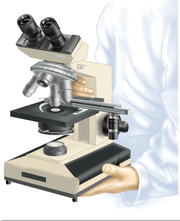
Figure 1.1 The microscope should be held firmly with both hands while being carried.
